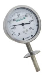
TEMPRESS gas pressure thermometer is made to meet the requirements of food and pharmaceutical industries.
